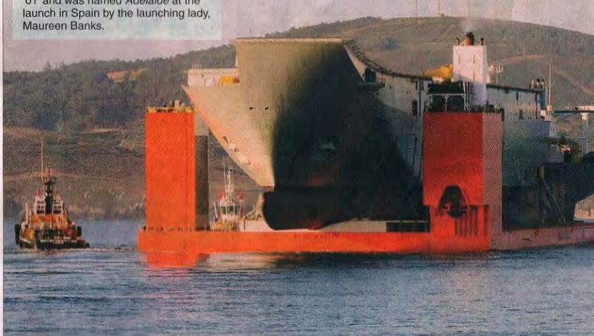
AUSTRALIA BOUND: The first hull of Navy's new amphibious ships departs from Ferrol in northern Spain. Right, the hull was loaded onto Blue Marlin in a significant engineering feat that involved submerging the heavy lift vessel so the hull could be floated onto it.
